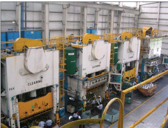
Tier 1 Automotive Stamping Plant Presses Retrofitted With Press Pac® Hydraulic Clutch/Brakes
