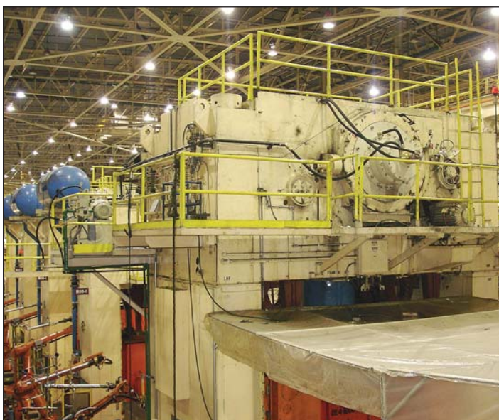
Press Pac® 2297 Separate Clutch & Brake Danly* 1600 Ton Double Action Stamping Press Installation
