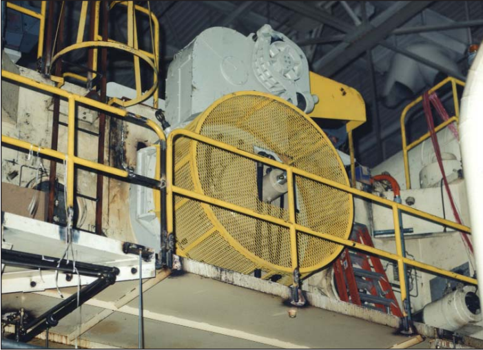
Press Pac® 2232 Separate Clutch & Brake Danly* 800 Ton Stamping Press Installation
