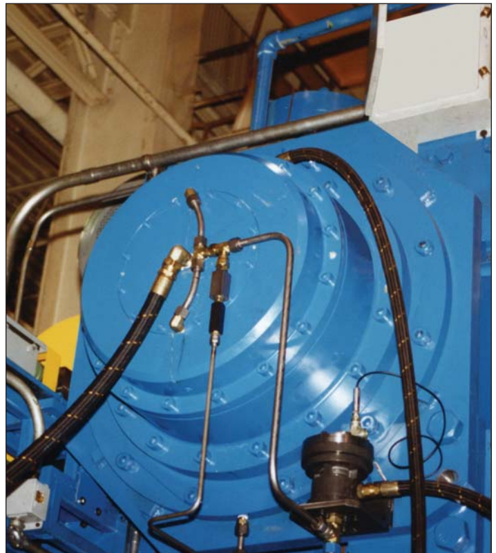
Press Pac® Brake Only Application Ajax® 1300 Ton Forging Press Application
