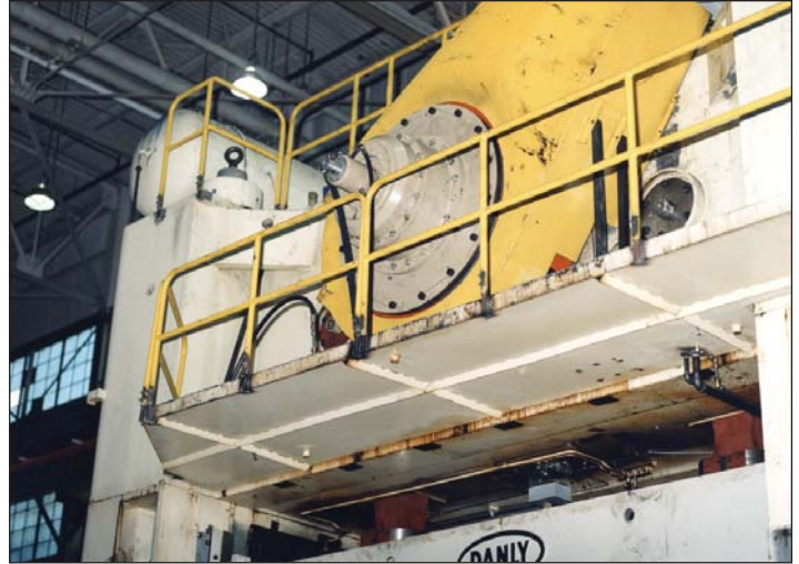
Press Pac® 2232 Separate Clutch & Brake Danly* 800 Ton Stamping Press Installation
