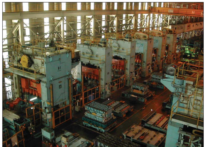
Automotive Stamping Plant Tandem Line Retrofitted With Press Pac® 2165 Units
