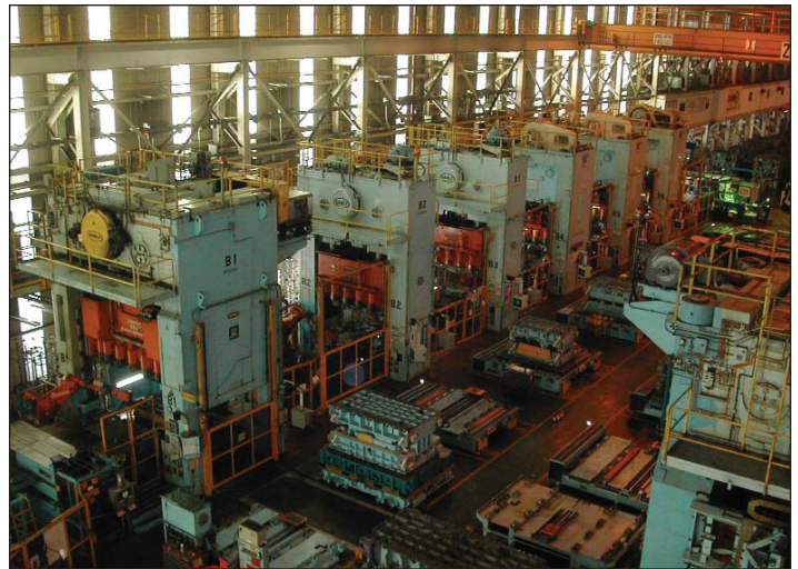
Automotive Stamping Plant Tandem Line Retrofitted With Press Pac® Hydraulic Clutch/Brakes
