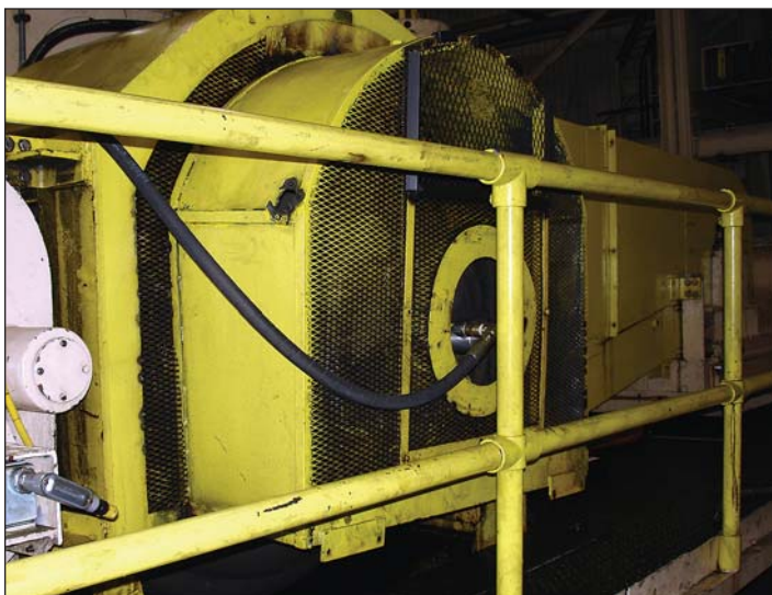
Press Pac® 3294 Series – Hydraulic Actuation / Oil Cooled
