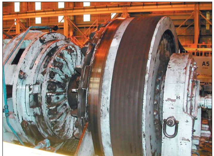
Dry Friction Pneumatic Clutch/Brake
